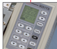
5031TS laminator control panel
