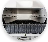
21.5" wide rubber conveyor belt removes shredded waste.
