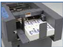
Automatic lift feed tray rids marking or misfeeding, as the vacuum feeding system and air knife compressor aid sheet separation.
