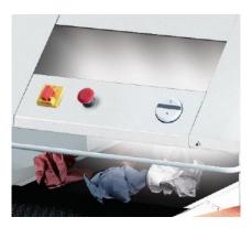
**ILLUMINATION OF THE WORKING AREA** The feeding area and the conveyor belt are illuminated by LEDs.
