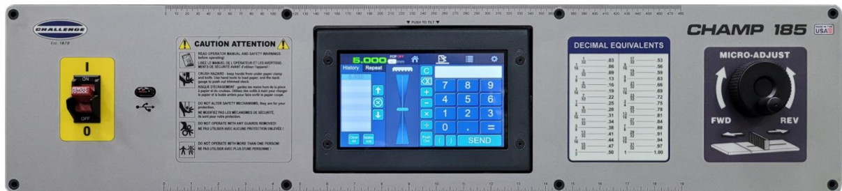
Figure 9 – Pro Control Console
