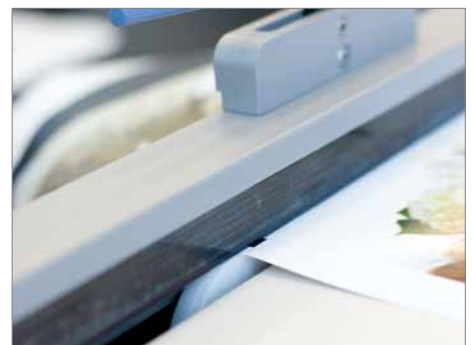
Creasing blade is visible, so it is possible to do precision creasing by visually aligning critical graphics with blade.
