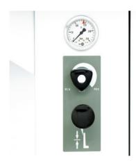
ADJUSTABLE HYDRAULIC CLAMP Clamping pressure is fully adjustable between 1,900 and 3,800 psi.
